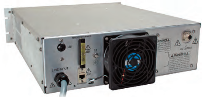
STA rear panel shown with local operation plug installed in 50 pin D connector
